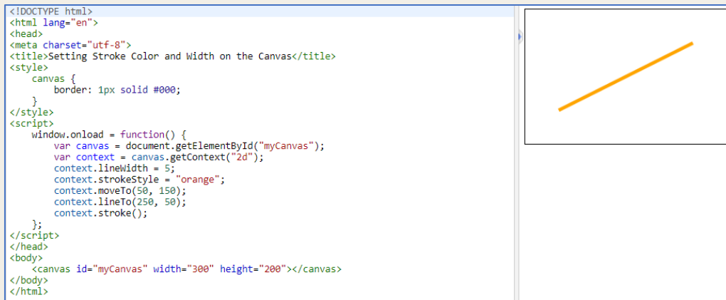
Figure 90 – Setting the styles and colours on stroke using strokeStyle and lineWidth properties (Source: https://www.tutorialrepublic.com/html-tutorial/html5-new-input-types.php )
