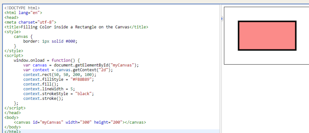
Figure 92 – Filling colour inside the canvas shapes by using the fillStyle() approach (Source: https://www.tutorialrepublic.com/html-tutorial/html5-new-input-types.php )
