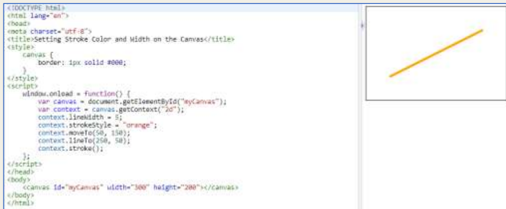
Figure 86 – Setting the styles and colours on stroke using strokeStyle and lineWidth properties (Source: https://www.tutorialrepublic.com/html-tutorial/html5-new-input-types.php )
