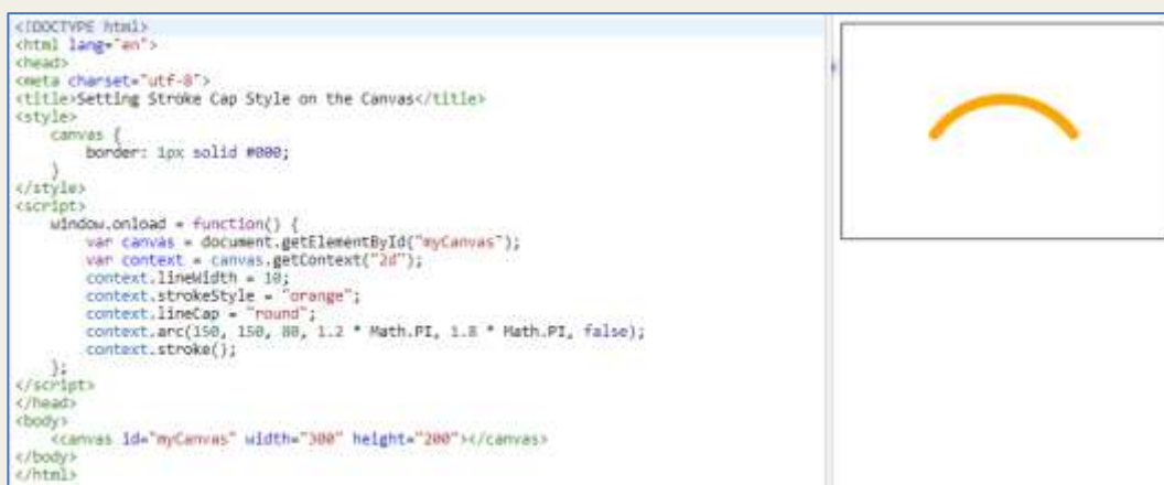
Figure 87 – Setting the cap style for the lines using the lineCap property (Source: https://www.tutorialrepublic.com/html-tutorial/html5-new-input-types.php )
