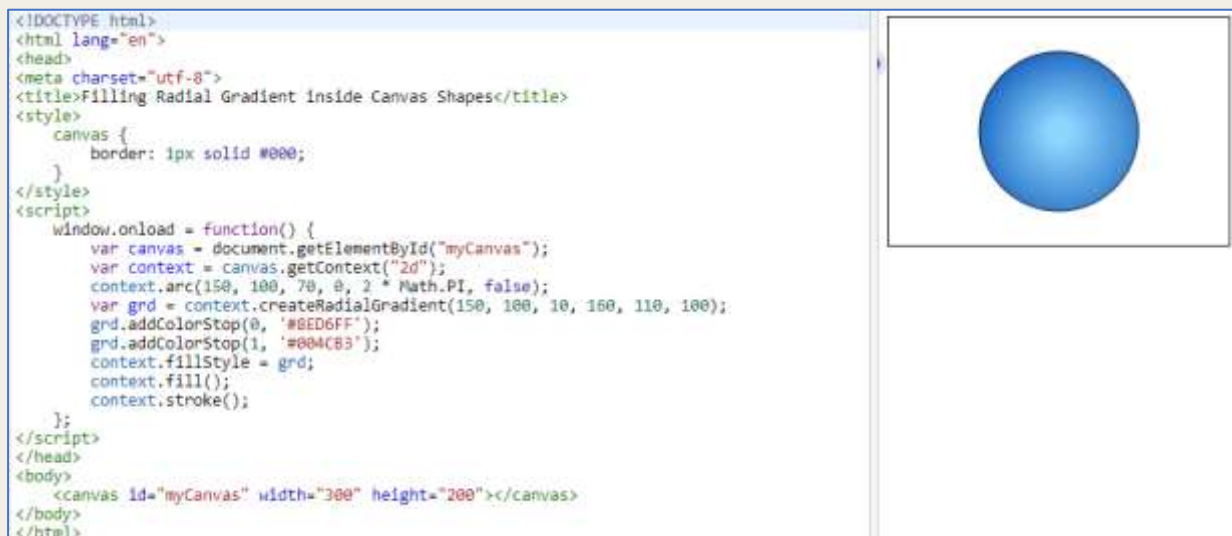
Figure 90 – Filling a radial gradient colour inside a circle through the createRadialGradient() method (Source: https://www.tutorialrepublic.com/html-tutorial/html5-new-input-types.php )
