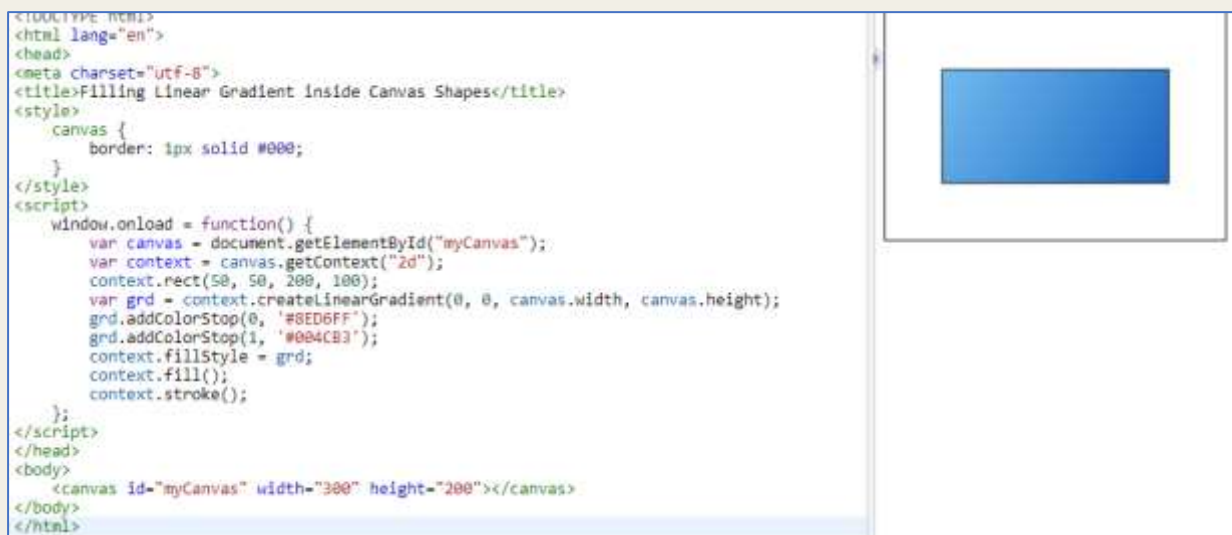
Figure 89 – Filling a linear gradient colour inside a rectangle using the createLinearGradient() method (Source: https://www.tutorialrepublic.com/html-tutorial/html5-new-input-types.php )
